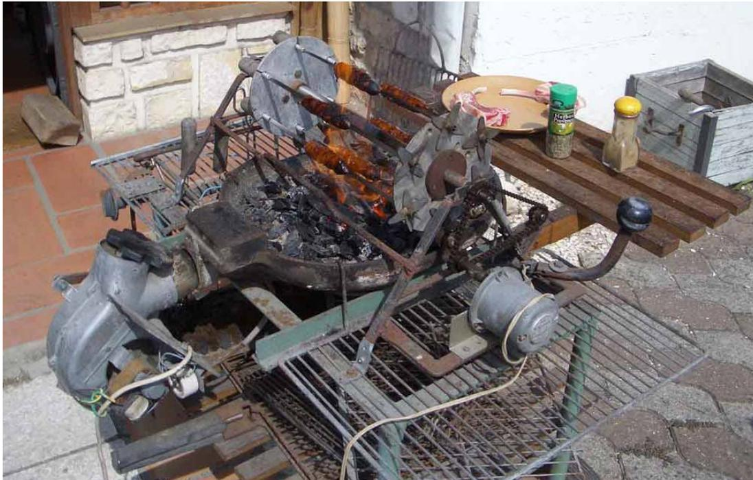
Composed of a rôtisserie engine, a chain from a Japanese photocopy machine, a fan from a kitchen ventilator, a forge from a forge-truck, various grates, lawn-mower wheels and a metal bed frame, the device features hand-made stainless steel skewers that rotate 1/4 of a turn every time they get to the bottom, so that the meat gets evenly cooked. I am stunned by its ingenuity and its nutty appearance. What a wonderful thing! Don’t you just want one?
